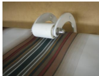
Pivot Bolt, Bracket is shown open
