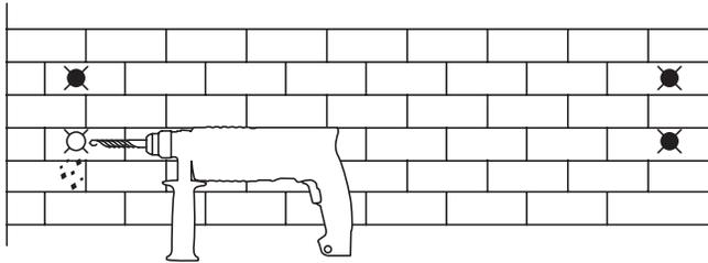
5. Gently tap the Sleeve Anchor into the hole. Ensure a minimum of 19cm (approx.3/4in.) remains outside the hole.
