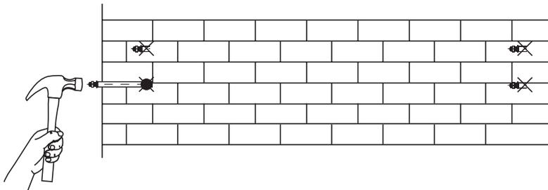
6. Install each Wall Bracket over each set of Sleeve Anchors, install the washer, lock washer and nut, then tighten.
