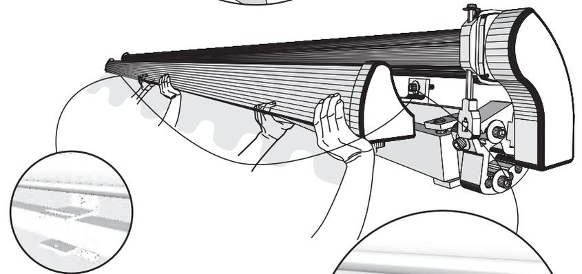
8. Insert the retaining bolt from the bottom as shown. Install the washer and nut, then tighten. CAUTION: MAKE SURE ALL NUTS ARE TIGHTENED.
