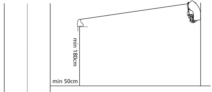
2. Ensure the surface can accommodate all three Wall Brackets within the dimensions shown below.
