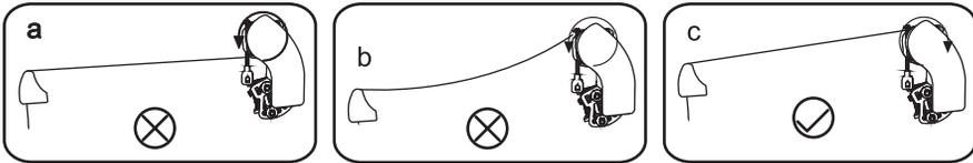
11. In the event that the awning does not open or close evenly it is generally due to the arms not being synchronized, as shown. This can easily be correctly and may require adjustment periodically. Simply loosen the Wrist Pin bolt (DO NOT FULLY LOOSEN OR REMOVE). This will allow the position of the Wrist Pin to be moved to the right or left very slightly so that the centre "elbow" aligns with the opposite arm. Once aligned, retighten the Wrist Pin nut.
