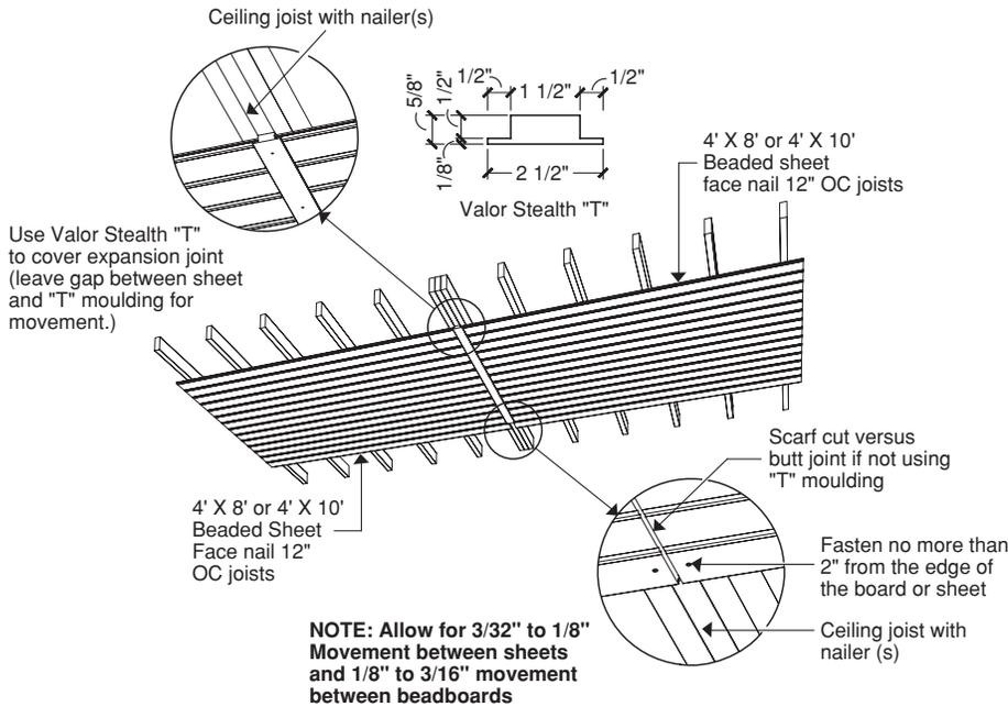
**Step 2:** Trim the first board before installing the first piece. Calculate how many boards it will take to cover the ceiling. Divide the width of the porch ceiling by the width of the beadboard to get the number of whole boards needed to cover the ceiling. If the last board is less than 2", trim down the first and last board to make the ceiling look evenly spaced.
